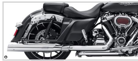
A. SCREAMIN' EAGLE HIGH-FLOW EXHAUST SYSTEM WITH STREET CANNON MUFFLERS **CHROME WITH CHROME MUFFLERS**
